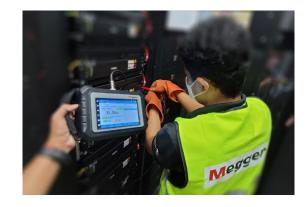
Figure 3: Testing of Individual Cell
